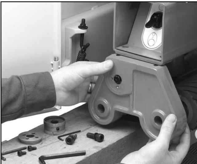
Figure 30. Work the casting off the roller shafts.
